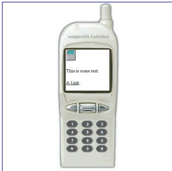
Figure 2. cHTML example inside waprofit's i-mode Phone Emulator. In cHTML, documents are structured like HTML documents.
