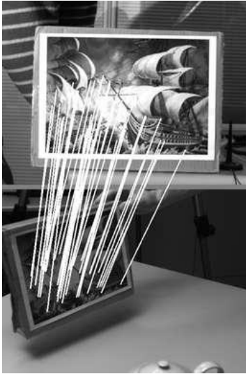
Figure 4. BazAR utilizes the Ferns algorithm to rapidly track surfaces without the need for fiducial markers [20].
