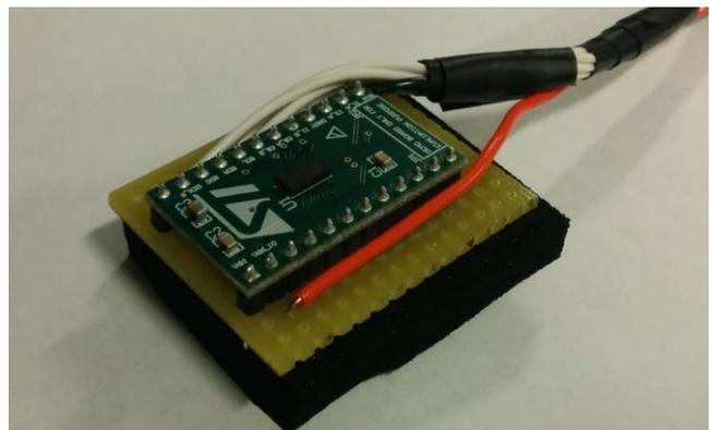
**Figure 1: The experimental SmartCube Inertial Measurement Unit**
