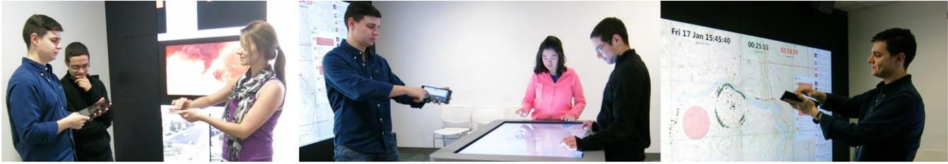
**Figure 2.** User performing “flick” gesture on iPad’s screen to send content from tablet to tablet (left); tablet to tabletop (center); and tablet to wall display (right).
